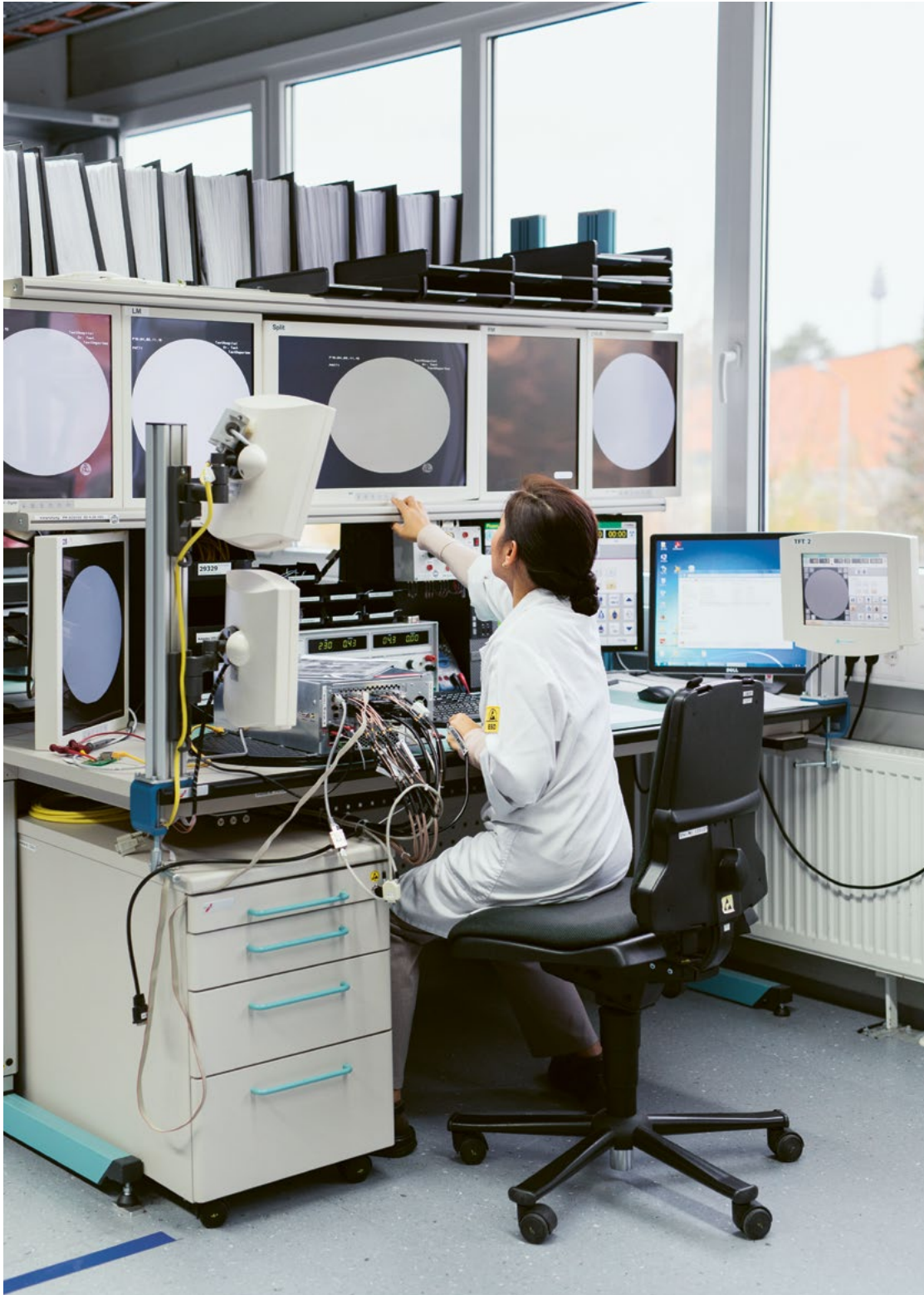
Testing and calibrating the monitors of the C-arm and mobile tripod are essential for reliable imaging in the operating room.
