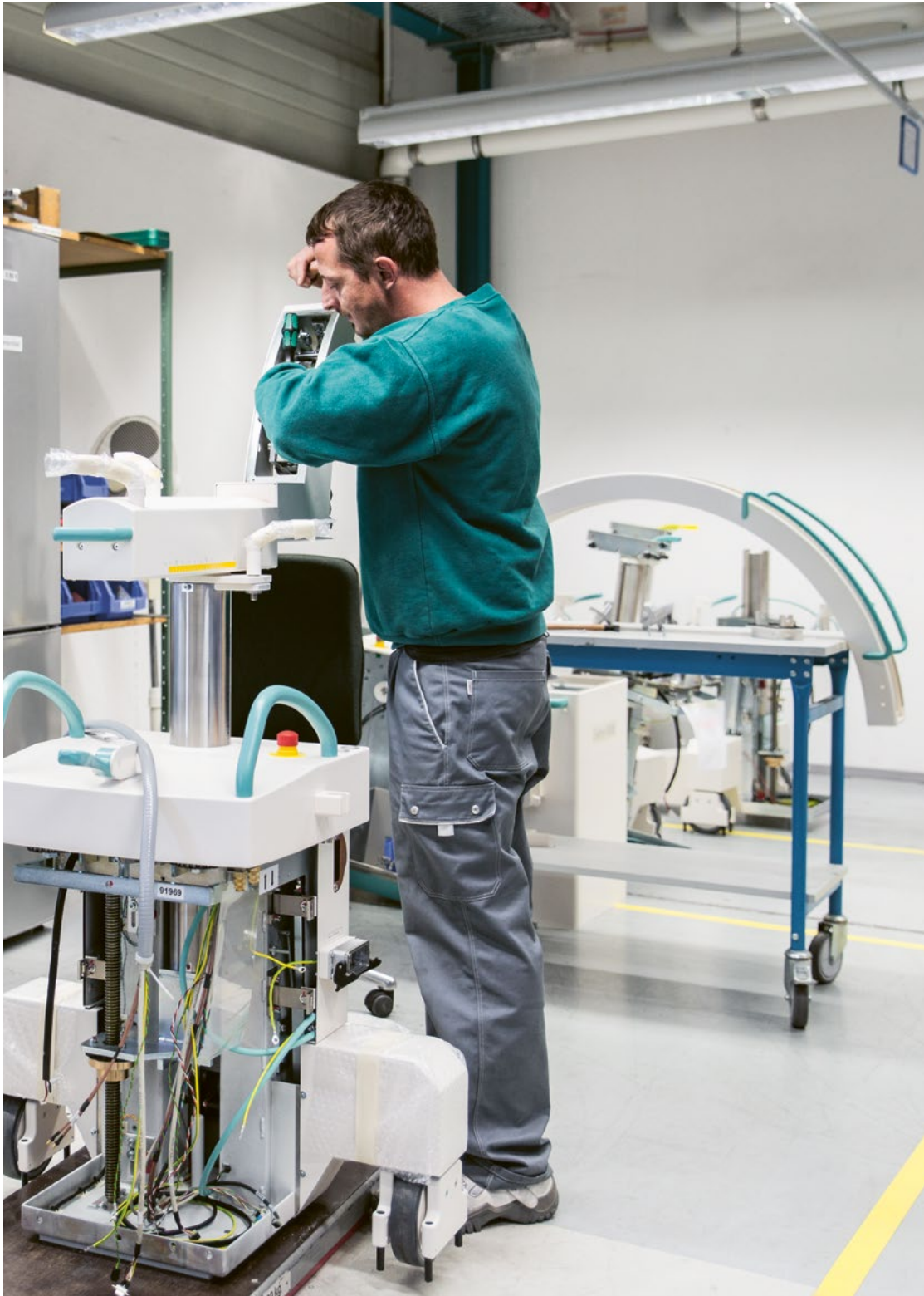
One employee is responsible for the assembly of a future C-arm, carrying out both the mechanical and electronic assembly of the mobile tripod.
